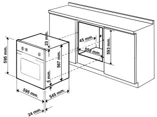
I The appliance must not come into contact with electrical parts once it has been installed. The consumption indications on the data plate have been calculated for this type of installation.
